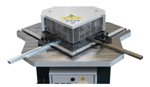
The many **T-slots on the bench** allow for the use of **mechanical and/or hide-away backstops** to perform **complex notching cycles**. To make your work easier still, set squares feature **reference holes every 15°.**
